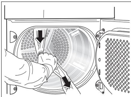
3. Remove foil hose and polystyrene padding from the machine.
